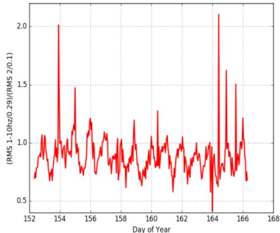
From ET requirement  $rms_{2Hz} = 0.1\text{nm}$  and  $rms_{1-10Hz} = 0.29\text{nm}$ .
