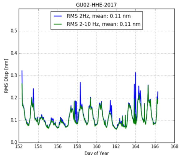
$rms_{2\text{Hz}}$  and  $rms_{2-10\text{Hz}}$  can be significantly different.
