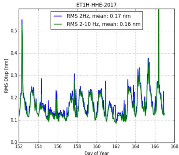
$rms_{2\text{Hz}}$  and  $rms_{2-10\text{Hz}}$  can be significantly different.
